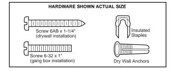
Figure 1 STANDARD INSTALLATION
